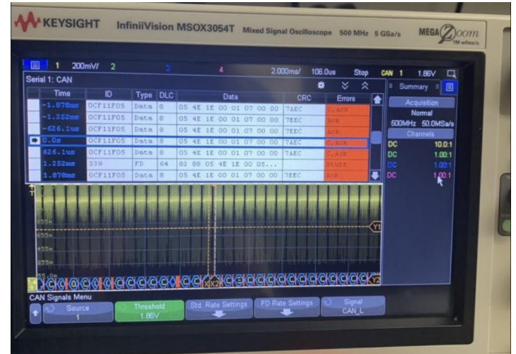
Keysight oscilloscope showing the CAN_L signal from the Kelly motor controller
